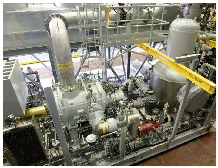
Screw compressor in Howden process gas package
