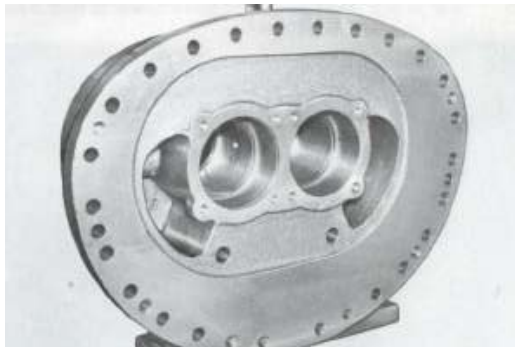
Fig. 043 After Removing Main Bearings
