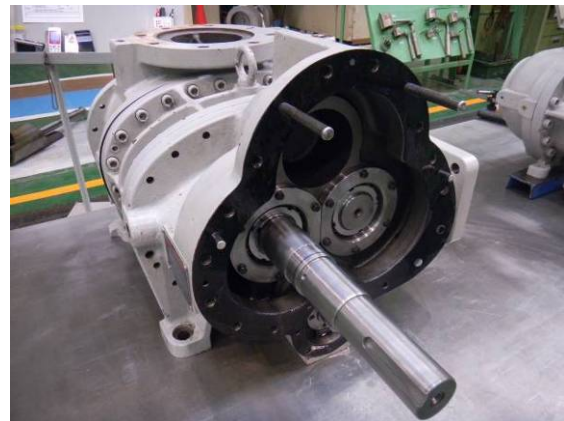
Fig. 026 After Bearing Cover Removal
