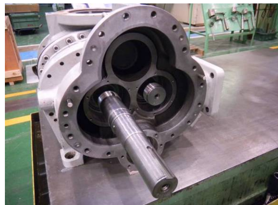
Fig. 046 After Removing Bearing
