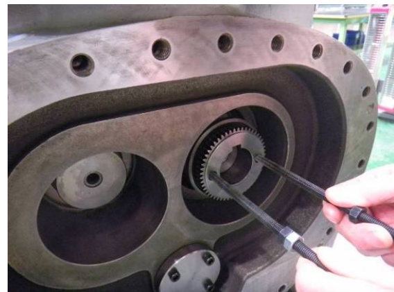
Fig. 047 Removing Drive Hub
