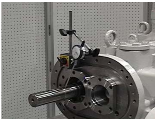
Check the runout of the male rotor shaft
