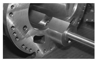
Pulling out the Unloader Slide Valve and Variable Auxiliary Slide Valve
