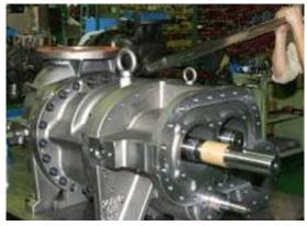
Tightening the Bolts using a Torque Wrench
