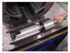
Separating the Unloader Slide Valve and Variable Auxiliary Slide Valve
