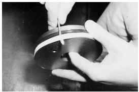
Removing the Cap Seal
