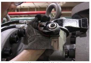
In case of Large sized Models, use a Hydraulic Torque Wrench
