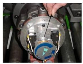
Loosen the Set Screw of the Micro Switch Cam
