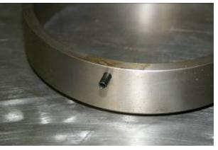
Type 2: Locked by a Spring Pin
