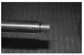
O-ring [63] at the tip of Unloader Push Rod
