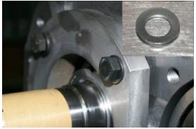
Removing the Thrust Bearing Gland
