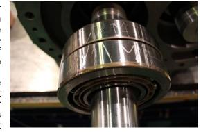
combine both bearings with the bearing number carving facing the outside of the machine. Then, use a blue whetstone to write the above "V" marking on the bearing to show the inside direction of the machine (see above picture). Then, install the bearing
