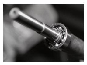
**Ball Bearing for the Indicator Cam**
