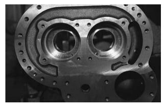
c) Install the O-ring [451] to the O-ring groove which located inside the hole to which is attached to the Vi adjusting rod of bearing head.
