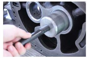
Aligning the Bearing position using Guide Bar
