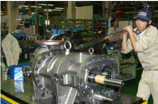
Fig. 3-86 Tightening Hexagon Head Cap Screws with Torque Wrench
