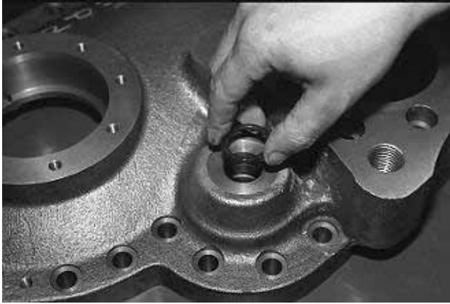
Fig.40 Bearing Cover Side “O” Ring of Vi Adjusting Rod
