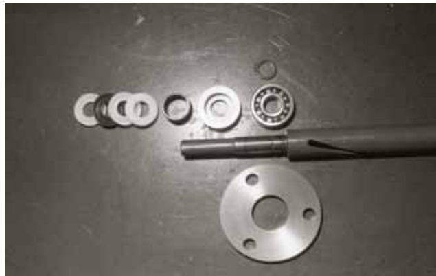
Fig. 3-25 Indicator Cam Seal Section Components
