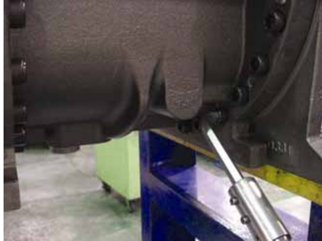
Fig. 3-4 Removing Lower Screws
