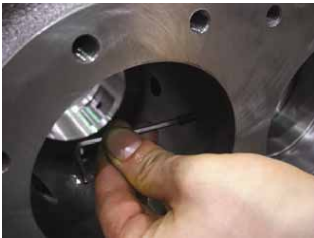
Fig. 3-35 Loosening the Balance Piston Locking Screw
