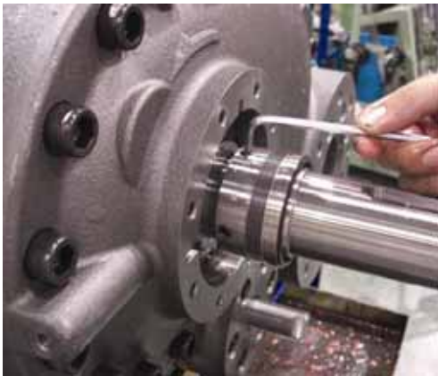
Fig. 3-9 Loosening the Set Screws on Seal Collar
