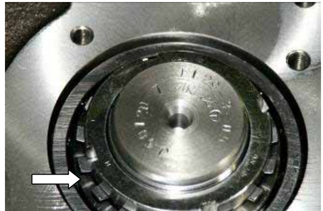
Fig. 3-93 Lock Washer Claws
