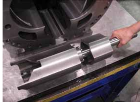
Fig. 3-61 Separating the Variable Vi Auxiliary Valve and Unloader Slide Valve
