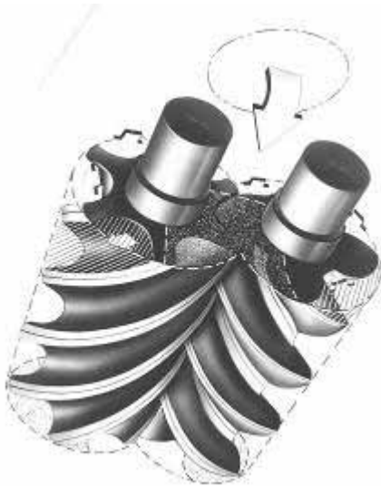
Fig. 1-6 Gas Suction Phase Is About to End
