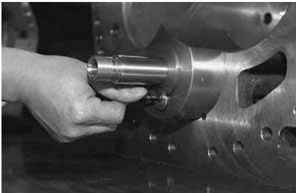
Fig. 3-58 Removing the Lock Washer (Products in and before 2003)
