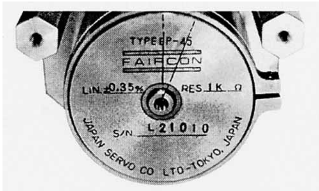
Fig. 3-130 Positioning Mark on Potentiometer
