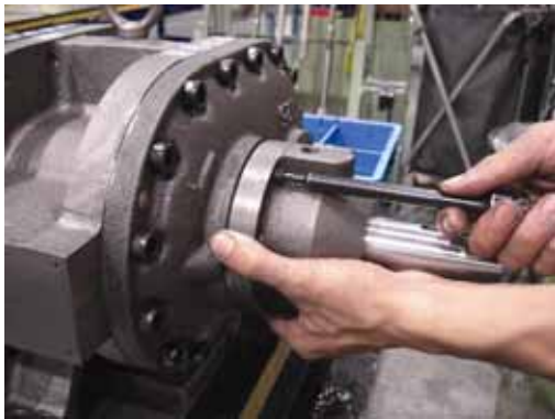
Fig. 3-7 Removing the Seal Cover
