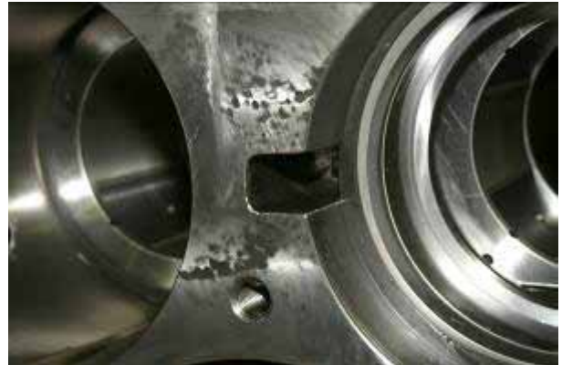
Fig. 3-34 Balance Piston Locking (Groove) – Type 2
