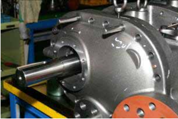
Fig. 3-104 Safety Bolts for Retaining the Bearing Cover
