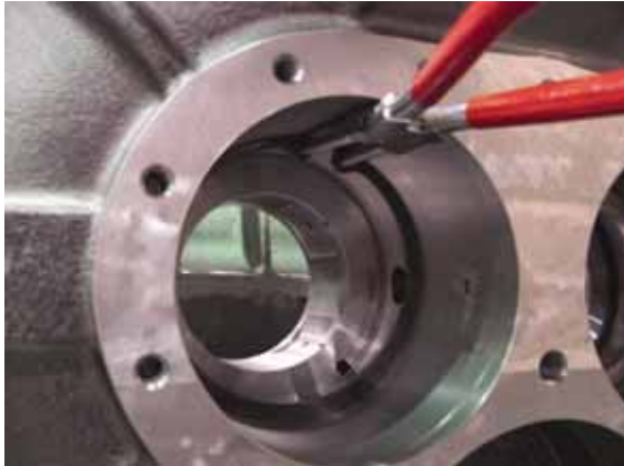
Fig. 3-54 Removing the Side Bearing Stop Ring
