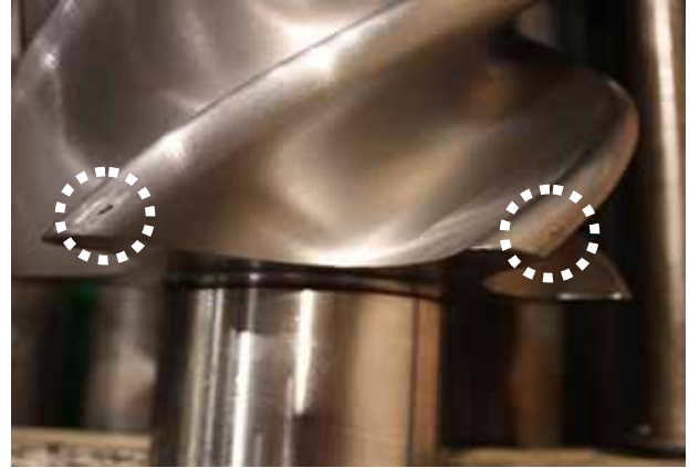
Fig. 3-75 Stamp Marks on Discharge Side Lobe End of Female Rotor
