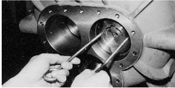
Fig. 3-32 Pulling Out the Balance Piston
