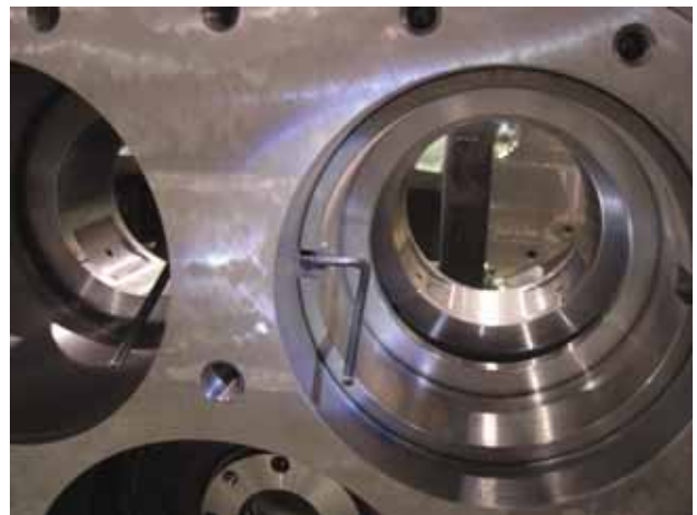
Fig. 3-35 Loosening the Balance Piston Locking Screw
