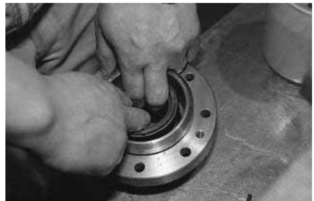
Fig. 3-122 Fitting the Mating Ring into Seal Cover
