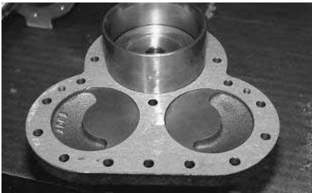
Fig. 3-110 Affixing the Gasket
