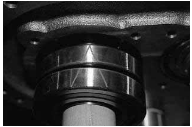
Fig. 3-89 V Mark on Thrust Bearing
