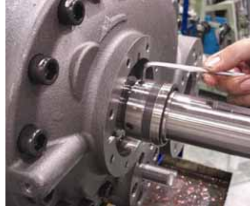
Fig. 3-120 Installing the Mechanical Seal Assembly(200 and 320 Models)
