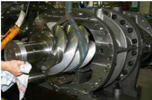
Fig. 3-76 Installing the Male Rotor
