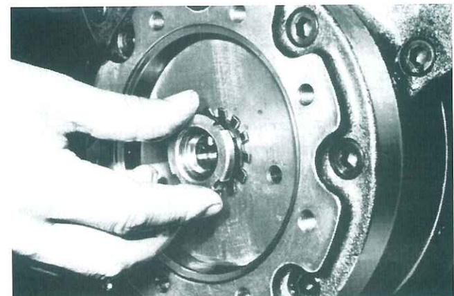
Fig. 138 Fitting washer and retaining nut
