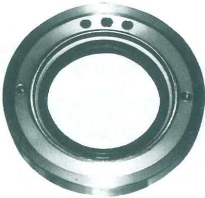
Fig. 146-1 Seal retainer & oil seal
