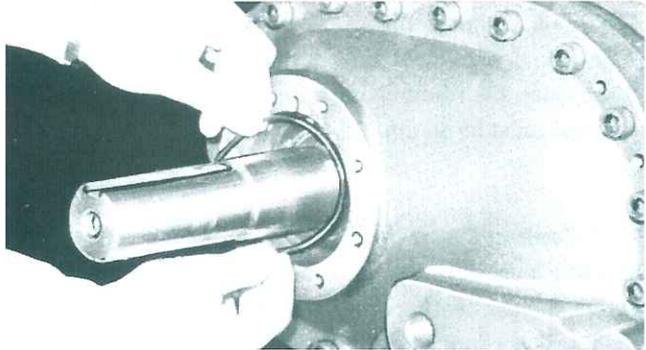
Fig. 149 Positioning "O" ring of seal cover
