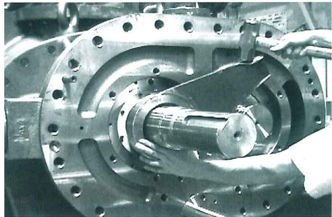
Fig. 116 (400) Fastening locknut
