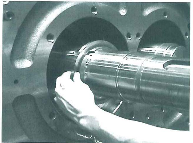
Fig. 400-21 Alignment spacer (2)
