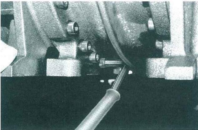
Fig.15 Lower Allen screws securing the suction cover
