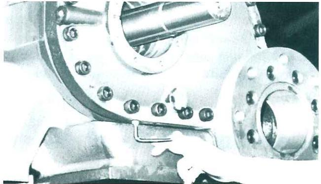
Fig.132 Do not forget the oil drain plug
