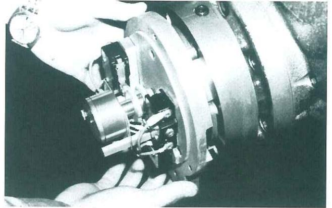
Fig. 33 Removing indicator
