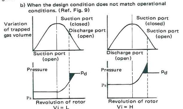
(1) In case of high compression ratio operation using a compressor with a small volume ratio.
