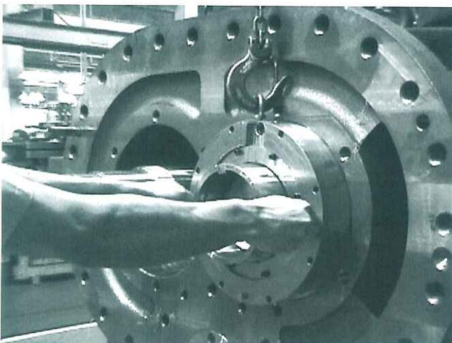
Fig.400-19 Thrust bearing (2)
