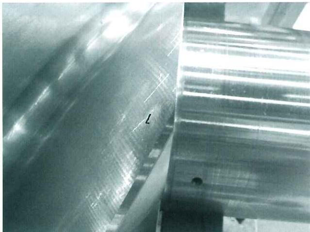
Fig. 86 Set marks of male rotor (400M)
