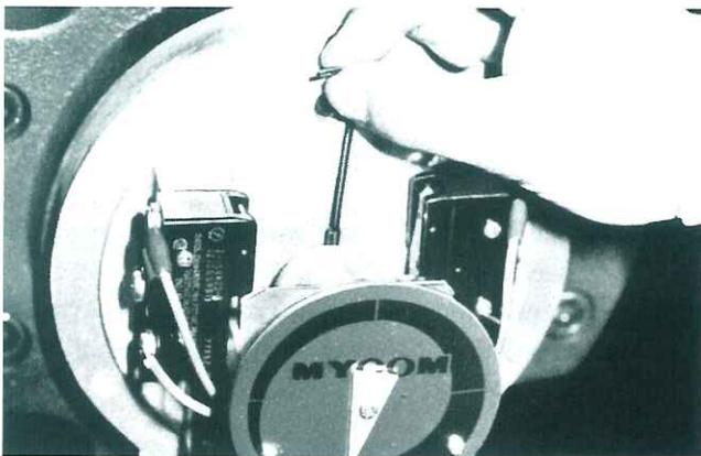
Fig.31 Loosening Allen screws holding cam shaft and micro-switch cam.
