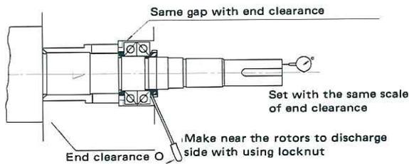
g) The same methods should be used for setting the end clearance of the female rotor. Please note however that in order to position the female rotor at the discharge side a screw driver must be used to shoving the rotor forward as shown in Fig 117.
