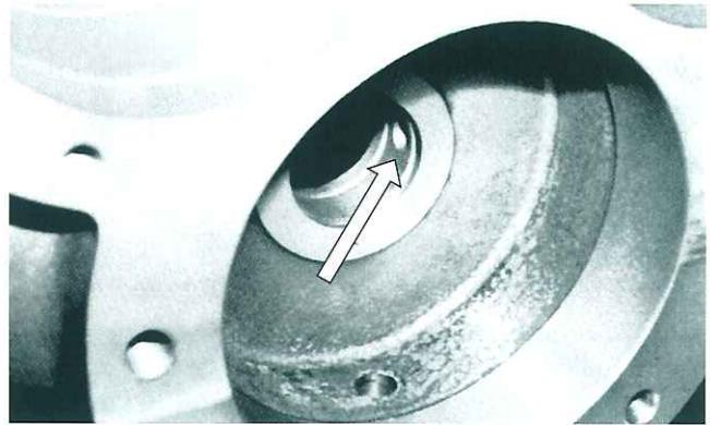
Fig. 69 Oil hole for injection
