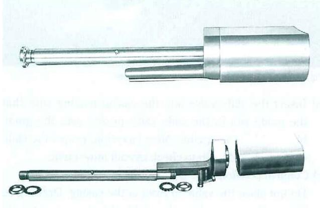
Fig. 78 Unloader slide valve assemblies (upper)
