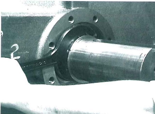
Fig.400-6 Lock nut sleeve (1)
