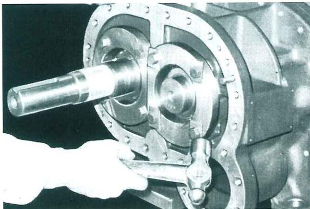
Fig. 123 Bending of out side of claw washer
