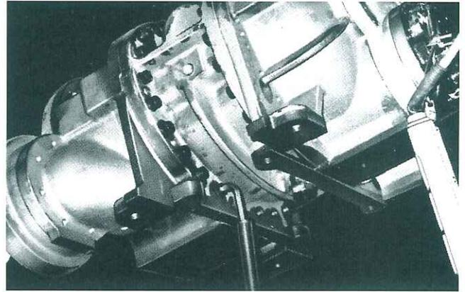
Fig.16 Lower Allen screws securing the bearing head
