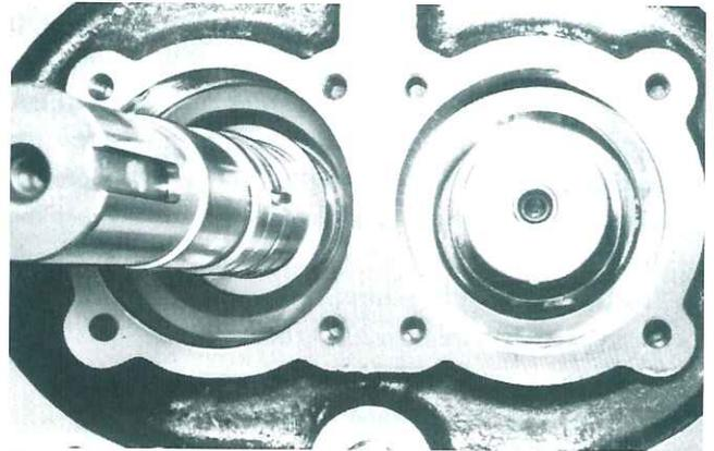
Fig. 54 Bearing spacer & washer after removed bearing
