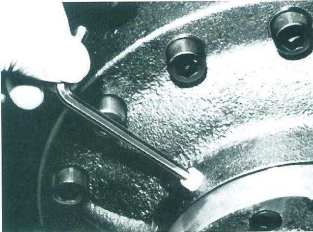
Fig. 152 Blind plug of bearing cover 160UD
