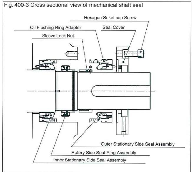
Fig. 400-3 Cross sectional view of mechanical shaft seal
