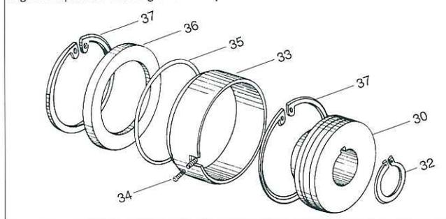
The balance piston (30) provides relief on the thrust bearing and the male rotor. For model 125LUD, the balance piston is positioned directly in the suction cover, while for the 160SUD model and lager there is a balance piston sleeve. The balance piston is crenulated (grooved) and forced fed
