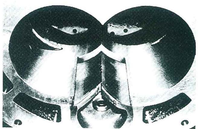
Fig. 79 Rotor casing and unloader slide valve
