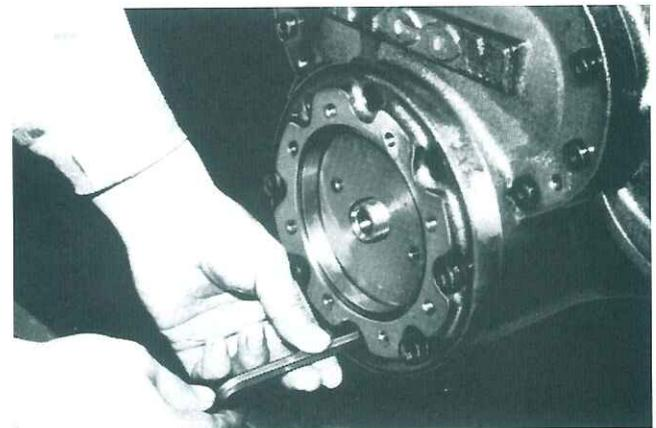
Fig. 137 Fasten cylinder and blind cover
