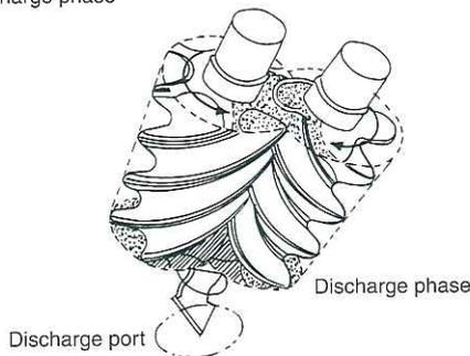
As described in the preceding passages, the screw compressor repeats suction, transfer, compression and discharge continuously at each lobe interface. This compressor has no valve mechanism as found in reciprocating compressors so no vibration or abrasion occurs. Moreover, stable, surge free running is performed under all operating conditions as this is a positive displacement type compressor.
