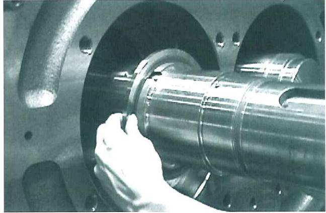
Fig. 114 (400) Setting bearing adjusting washer
