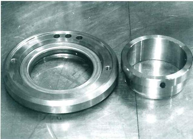
Fig. 146-2 Seal retainer oil seal and sleeve (2003 May~)
