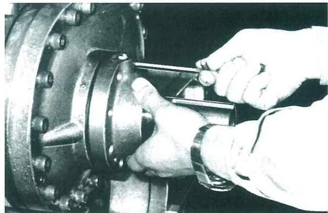
Fig 21 Removing Allen bolts securing seal cover
