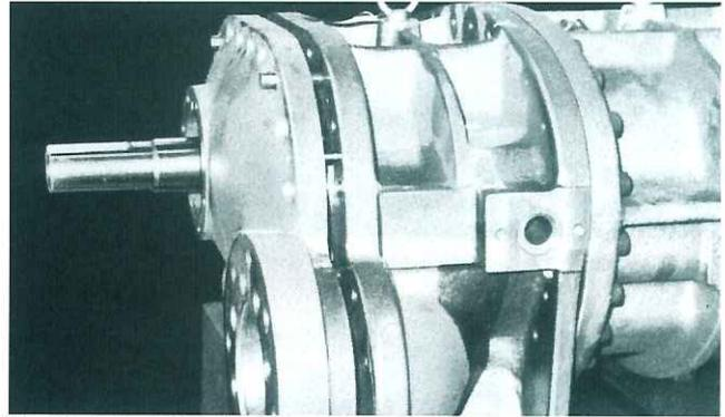
Fig.131 Setting of bearing cover
