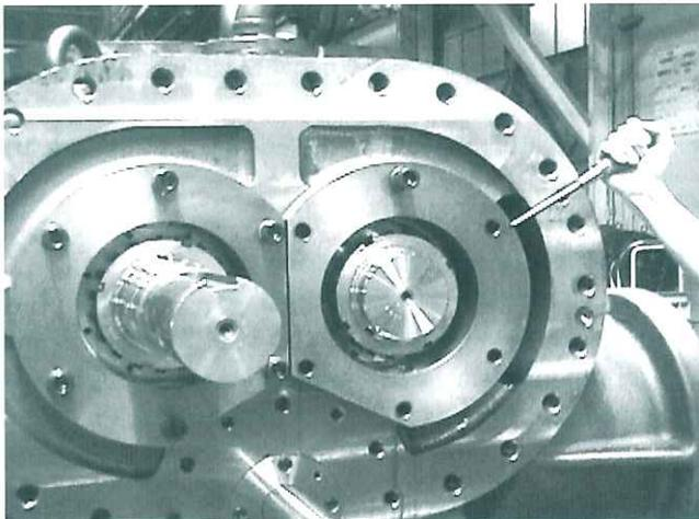
Fig. 400-13 Thrust bearing gland (1)
