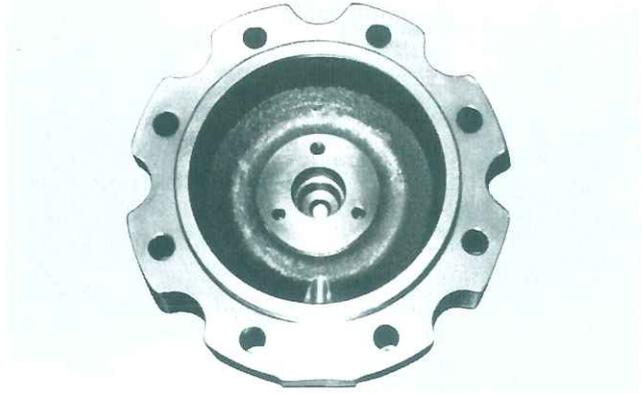
Fig. 39 Body of unloader cover
