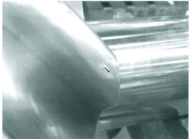
Fig. 87 Setting marks of female Rotor (400M)
