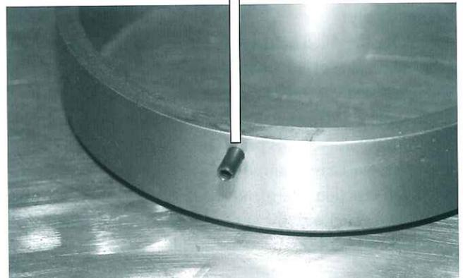
Fig.65 320&400UD Balance piston sleeve locking pin
