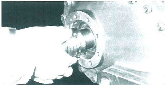
Fig. 150 Fitting seal assembly
