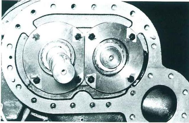
Fig. 50 Parts of thrust bearing gland (160UD)
