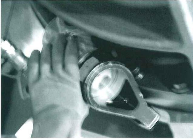
Fig. 102 Fastening of bolts by hydraulic wrench (320-400UD)
