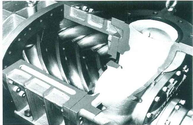
Fig.2 Rotation and compression by rotor
