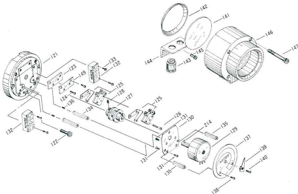
Fig. 156 Exploded view of unloader indicator (160SUD-250LUD)
