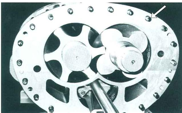
Fig. 92 Setting bolts of suction cover
