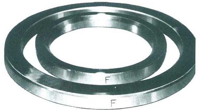
Fig. 55 Marks on the spacer and washer Disassembly of thrust bearing
