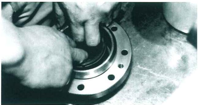
Fig. 151 Mounting carbons insert
