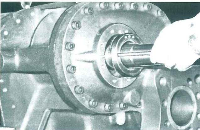
Fig. 147 Fitting seal retainer
