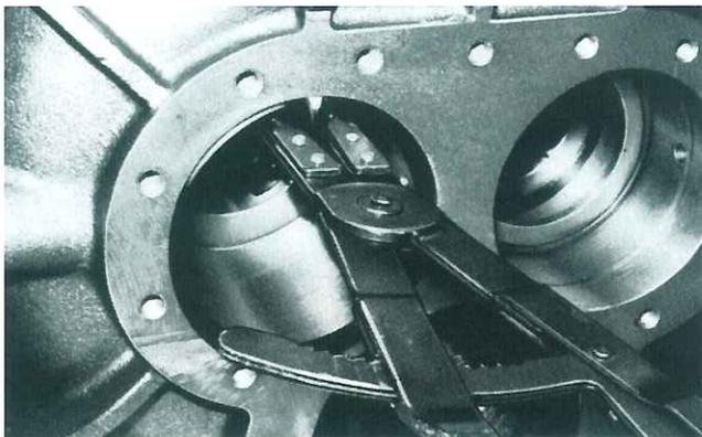
Fig. 91 Stop ring of side bearing
