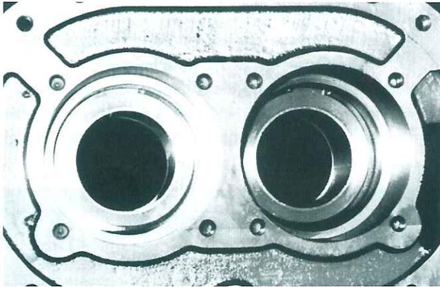
Fig. 84 Appearance of correctly installed main bearing
