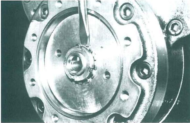
Fig. 140 Bending the claw washer
