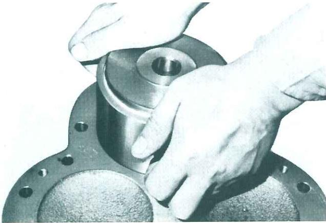
Fig. 133 Pushing piston into unloader cylinder
