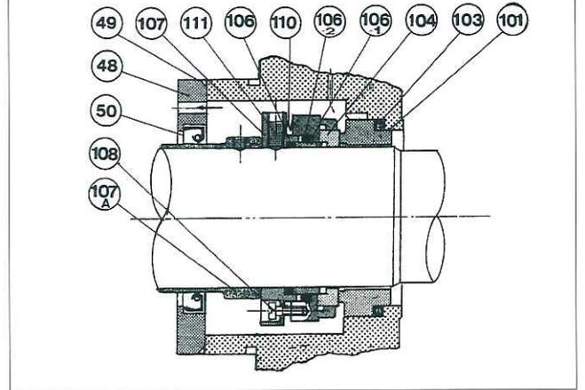
Fig. 145-2 Cross sectional view of component (Before May 2003)
