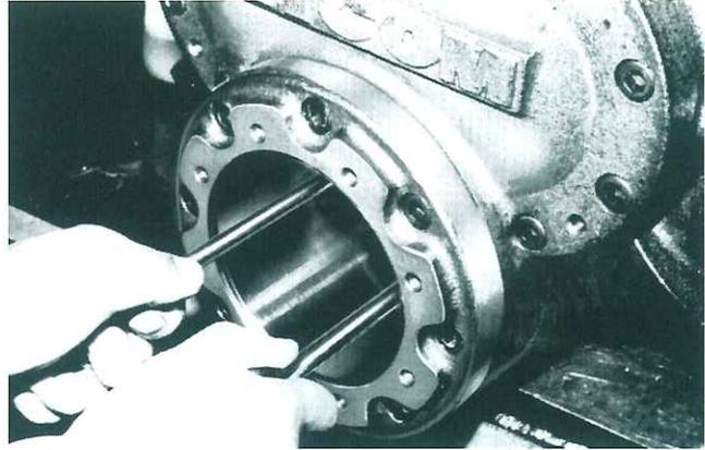
Fig. 142 Full unloader position (push to the end)
