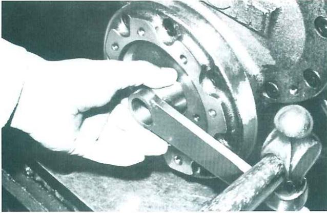
Fig. 139 Fasten the nut tightly
