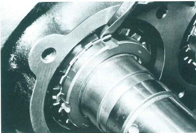
Fig. 122 Bending the claw of washer
