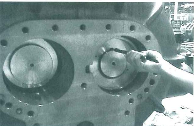
Fig. 103-2 Set the snap ring of the balance piston (400VMD)
