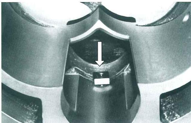
Fig.81 Guide block in the rotor casing
