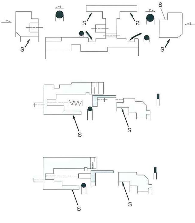
13. Apply lubricant to point S of the seal ring, and push in the ring evenly with the pin hole of the spring retainer aligned with the pin position of the driver collar.
