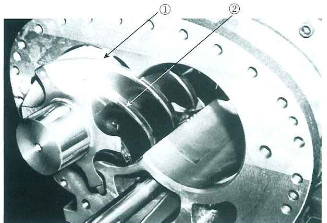
Fig. 88 Setting female rotor (200S)
