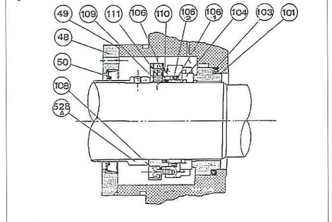
Parts of mechanical seal
