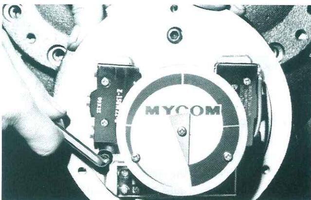
Fig. 32 Loosening Allen screws of micro-switch base plate
