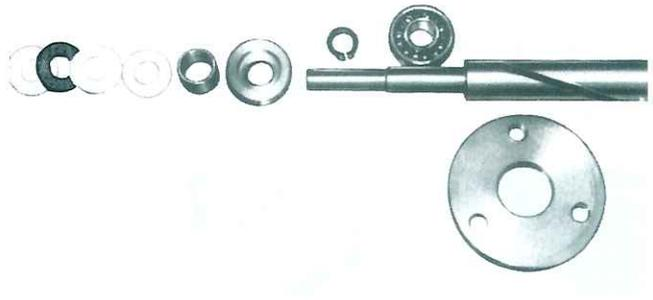
Fig. 40 Shaft seal parts of indicator cam
