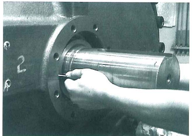
Fig. 400-8 Rotary side seal ring assembly
