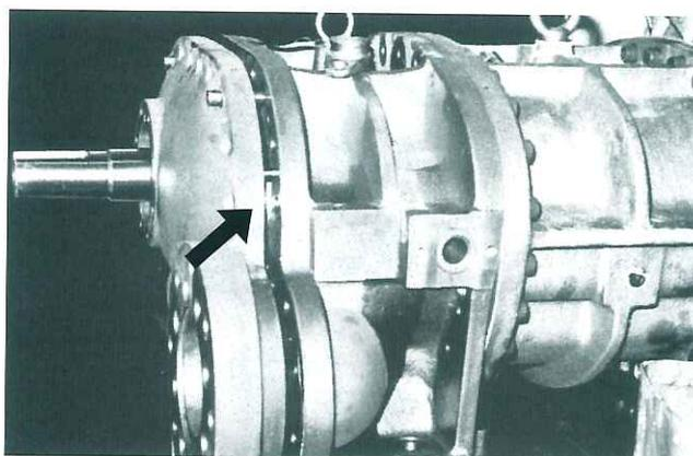
Fig. 45 Removing bearing cover
