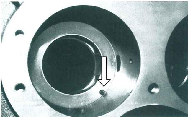
Fig. 90 Side bearing stopper
