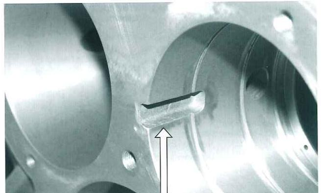
Fig.64 320&400UD Balance piston sleeve locking pin
