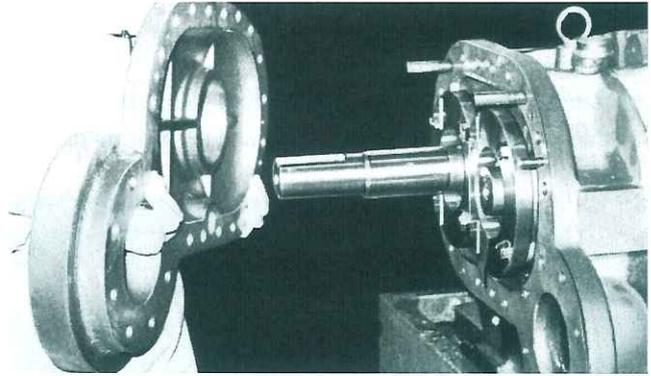
Fig. 130 Installing bearing cover
