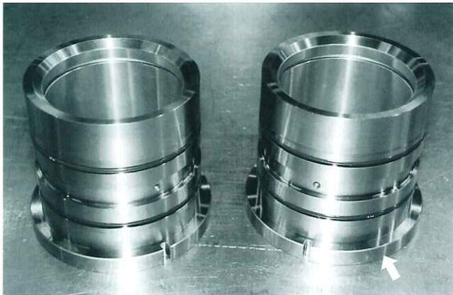
Fig. 85 Notch in bearing
