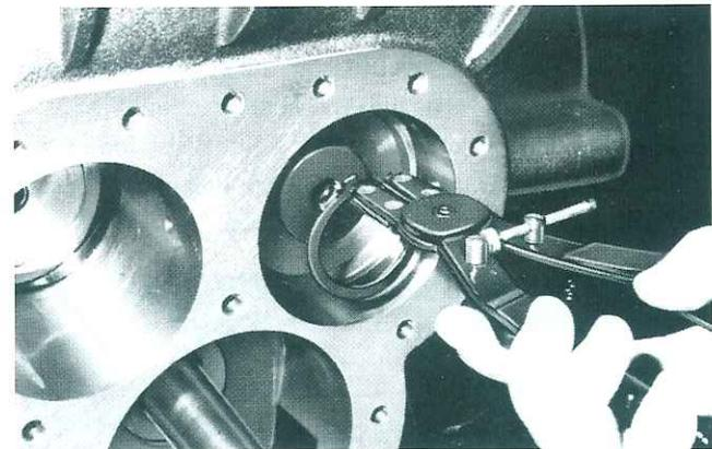
Fig.57 Removing snap ring holdings balance piston
