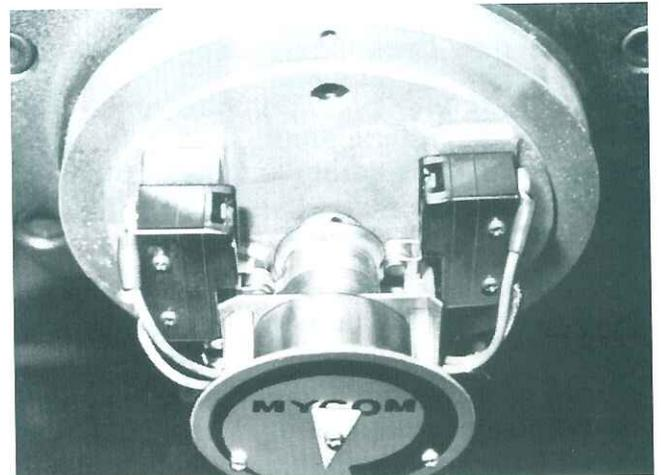
Fig.159 No load positioned cam in case of two micro-switch
