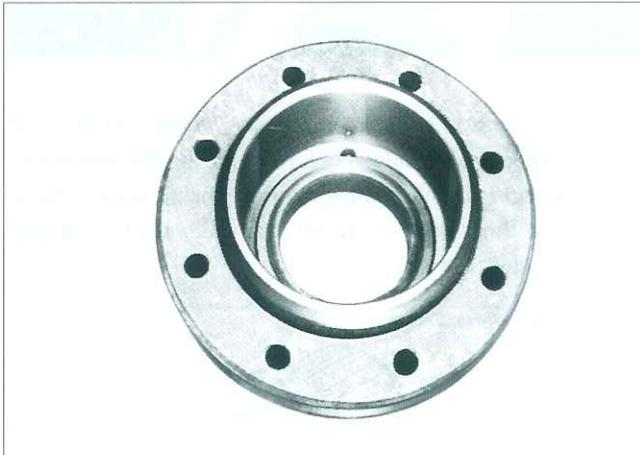
Fig. 28 Seal cover and carbon insert
