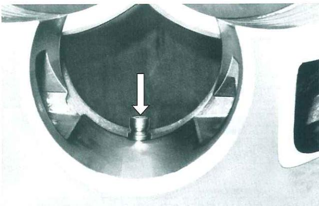
Fig. 80 Guide block stem inside of casing
