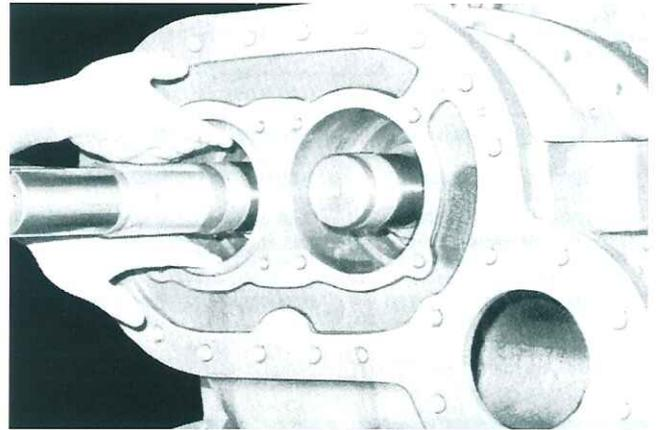
Fig.108 Setting thrust bearing spacer
