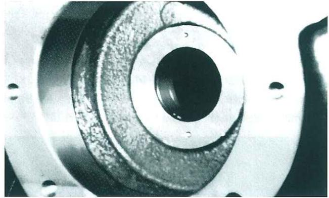
Fig. 68 Oil injection pipe gland
