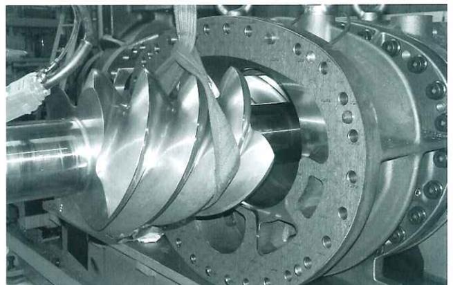
Fig. 89 Setting male rotor (400M)
